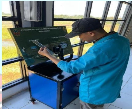
Gambar 2. 21 Memompa Tekanan Injector Tester
