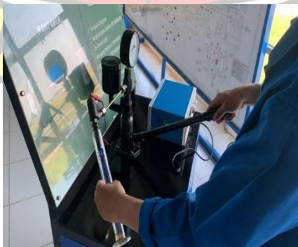
Gambar 3. 16 Memompa Tekanan Injector Tester
