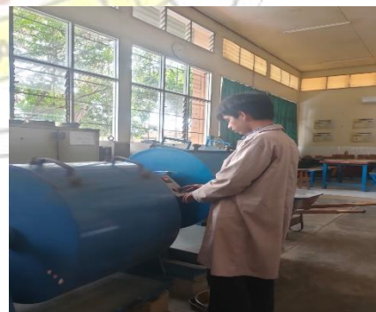
Gambar 11.6 Setting putaran sebanyak 500 (ABCD) 1000 (EFG)
