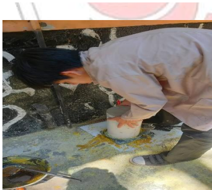
Gambar 12.9 Capping sampel beton
