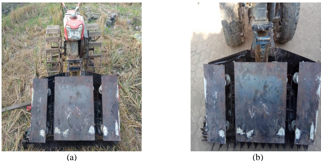
Figure 9. (a) Rice Cutting Machine Assembly (b) Rice Cutting Machine Connection Mounted on tractor farmer
