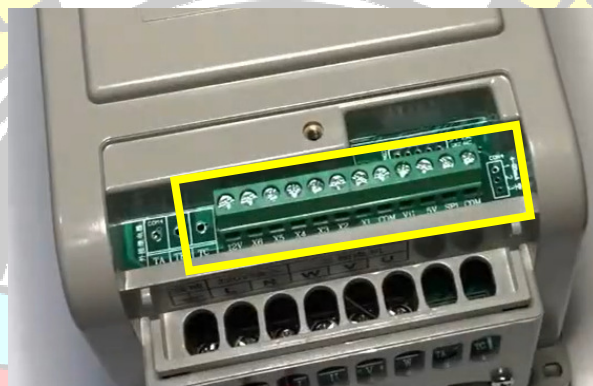
Gambar 2. 20 Terminal DC VFD
