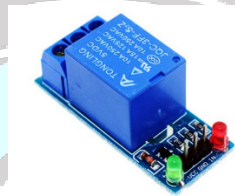
Gambar 2.13 Relay (Sumber: Zanoor, 2024)
