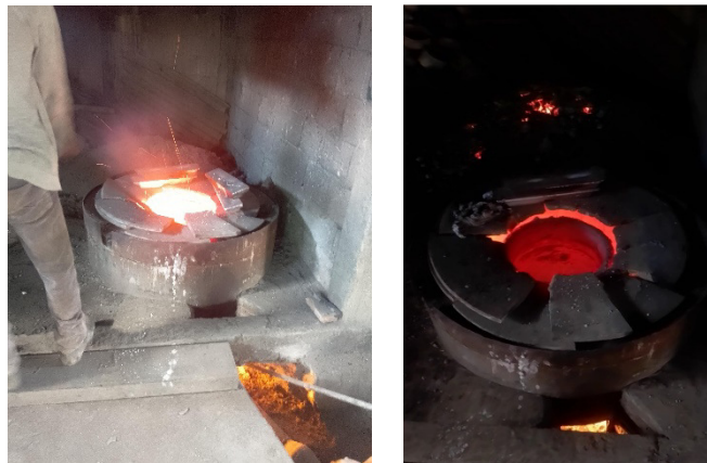
Gambar 3. 34 Proses Peleburan Aluminium
