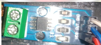
Gambar 2.11 Sensor Arus ACS712
