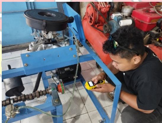
Gambar 4.6 Mengukur putaran camshaft
