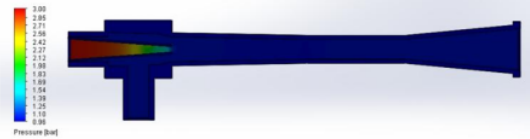
Fig. 6 Pressure contour with the suction diameter (d=20 mm)
