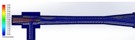
Fig. 9 Streamline with suction diameter (d=15 mm)
