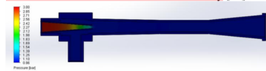
Fig. 2 Pressure contour with the suction diameter ( d=10 mm)
