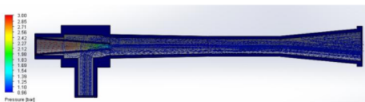
Fig. 10 Streamline with suction diameter (d=20 mm)
