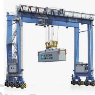
Gambar 2.2 Rubber Tyred Gantry
