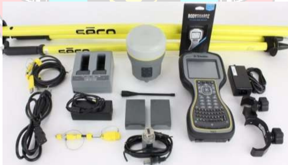
Gambar 2.8 Satu Set Trimble R10 GNSS GPS Receiver Kit Sumber : (Trimble R10 GNSS GPS Receiver Kit, 2023)
