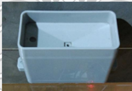
Gambar 2. 3 Tipping Bucket (Sumber: Prayogo, 2019)
