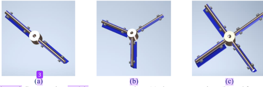
Figure 2. Pressure plate models: two pressure plates (a), three pressure plates (b), and four pressure plates (c).
