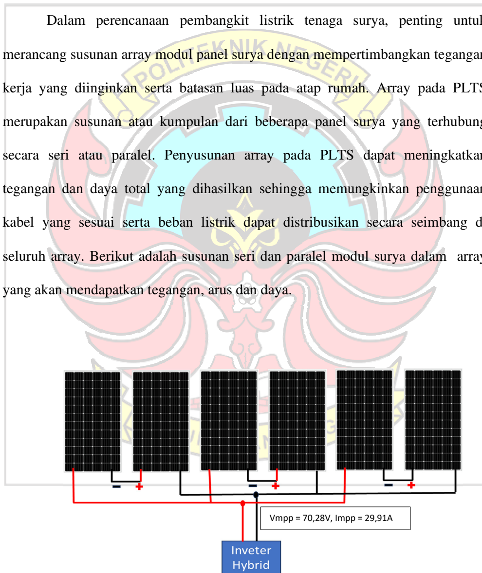
Gambar 4.9 Array Panel surya
