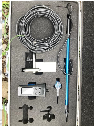
Gambar 2.7 Current Flow Meter
