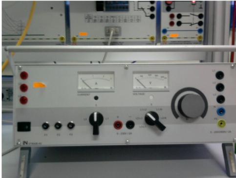
Power Supply 3 Phasa
