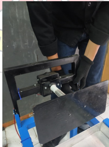
Gambar 4.10 Proses perakitan trigger limit switch
