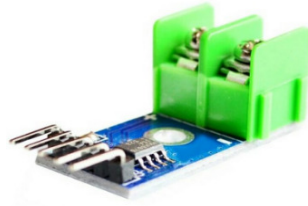
Gambar 2.26 Sensor Max 6675 (Sumber: https://shopee.co.id )
