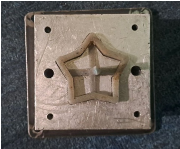
Mold Terisi Material HDPE
