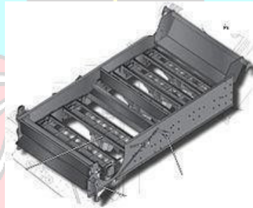
Gambar 2. 9 Pengayakan Vibrating Screen
