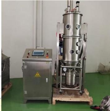
*Gambar 2.2 batch dryer*
