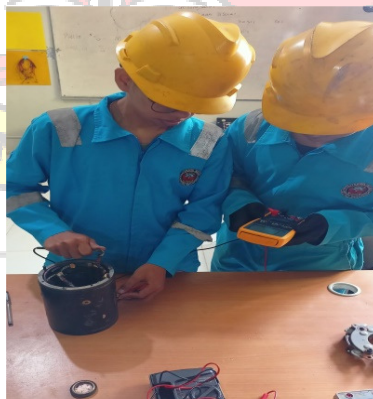
Gambar 4.11 Field winding ground test
