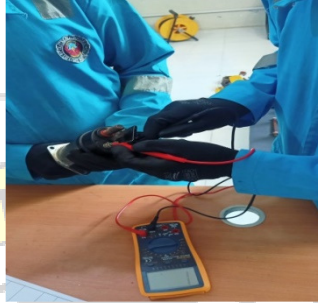
Gambar 4.21 Pengujian pull in coil
