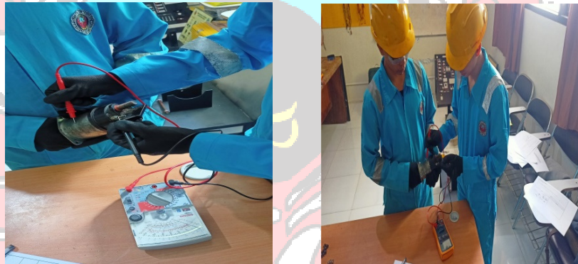
Gambar 4.9 Pengujian hold in coil
