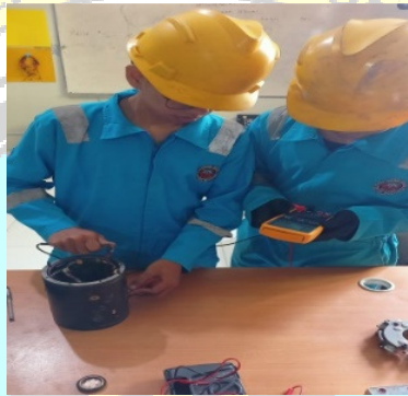
Gambar 4.24 Pengujian ground stator
