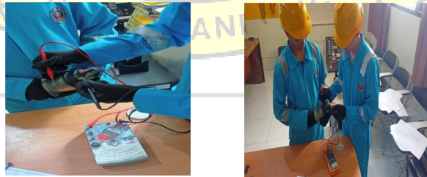
Gambar 4.22 Pengujian hold in coil
