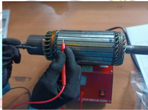
Gambar 4.26 Pengujian ground armature
