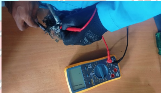
Gambar 4.19 Pengujian brush holder
