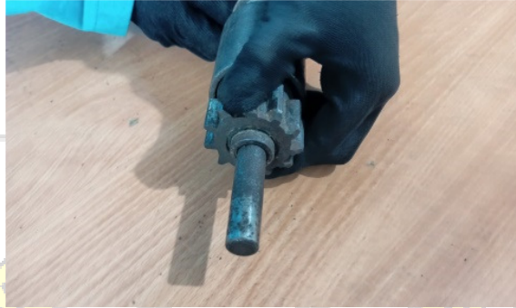
Gambar 4.32 Pengujian pinion drive
