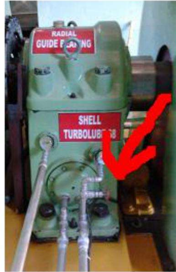
14. Buka valve pipa cooling water
