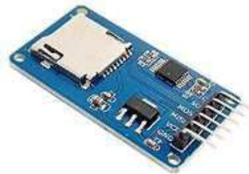
Gambar 2.17 Modul Micro SD Card Adapter Sumber : www.amazon.de
