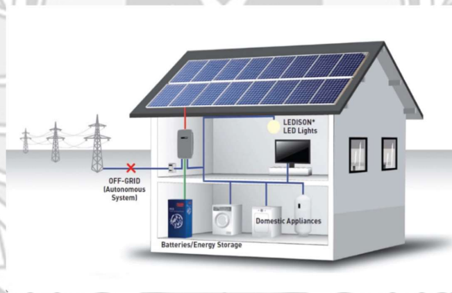
Gambar 2.4 Instalasi SHS Off Grid
