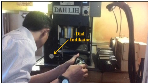
Figure 8. Turbine casing measurement process
