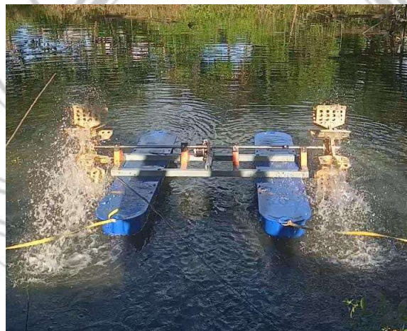
Gambar 4.2 Konstruksi Mekanik Aerator Peddle Wheel
