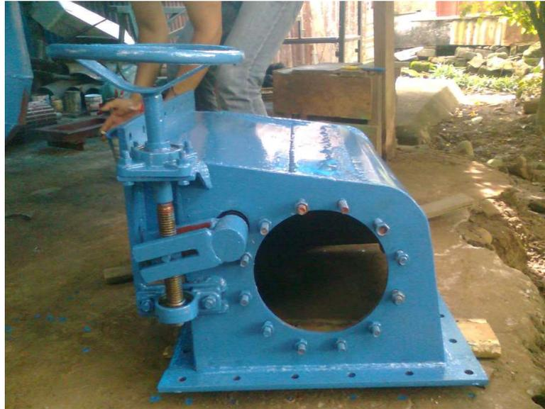
**Gambar 9. Casing turbin tampak samping kanan**
