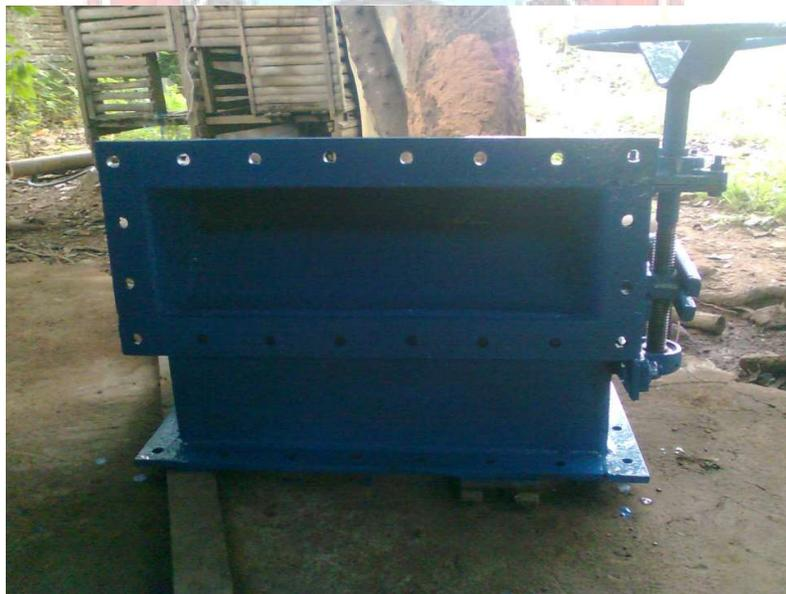
**Gambar 10. Casing turbin tampak depan**
