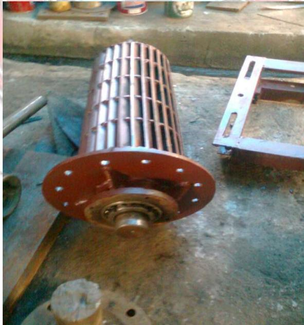
**Gambar 14. Turbin crossflow**
