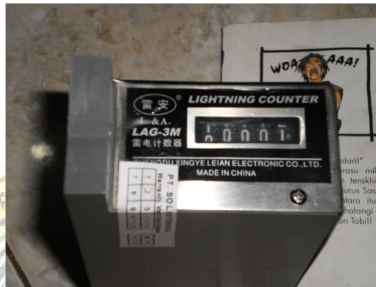
Gambar 15. Lightning Surge Counter (Recorder Petir)
