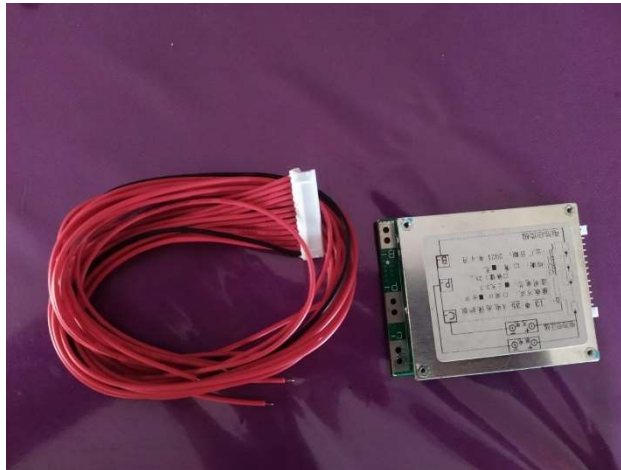
Gambar 2.8 BMS ( battery management system )
