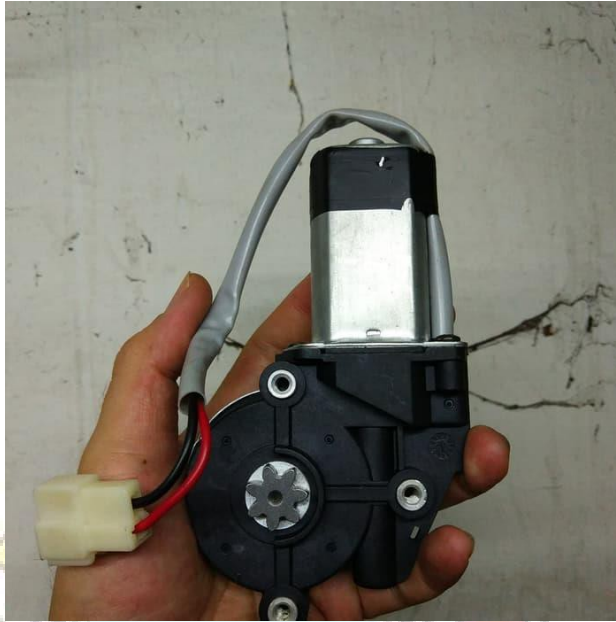
Gambar 2.15 Motor DC Power Window
