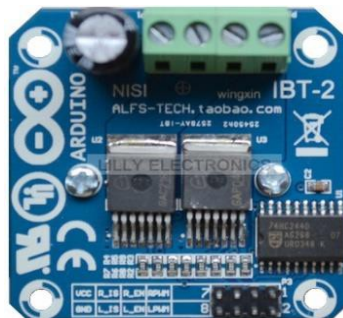
Gambar 2.19 Driver Motor BTS7960 / IBT-2
