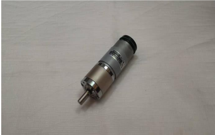
Gambar 2.16 Motor DC Planetary (PG45)
