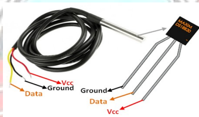
Gambar 2. 10 Sensor suhu DS18B20
