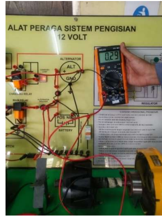
Measure Current of System by Removing Negative Battery Cable
