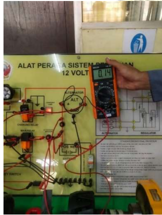
Test Output Current of Alternator Below 0.015A
