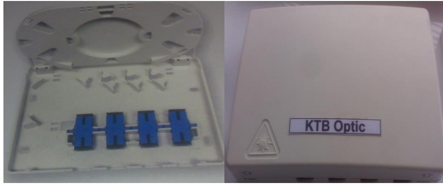
Gambar 2.13 Optical Termination Premises (OTP)
