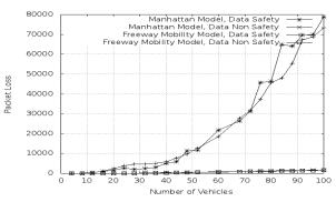
Fig. 9. Variation of packet loss with number of simulated vehicles
