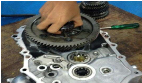
Gambar 3.16 Melepas case diferensial assembly
