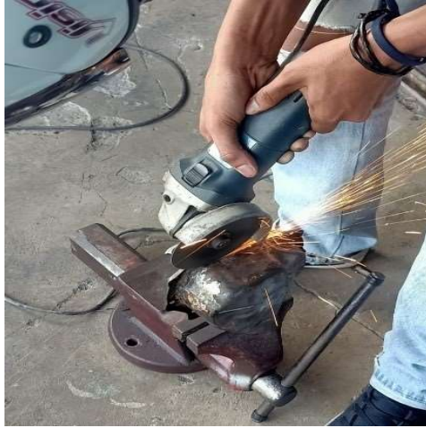
Gambar 3.18 cutway cover sub-assembly case transmisi manual
