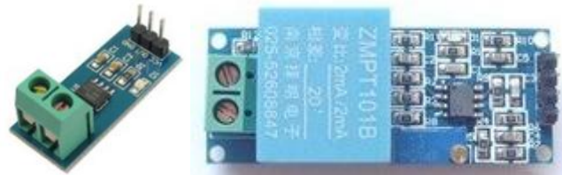
Gambar 5.4. Sensor Arus ACS712 & Tegangan ZMPT101B
