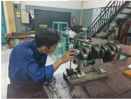
Gambar 18. Pengukuran runout crankshaft
