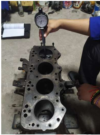
Gambar 16. Pengukuran linear bore
