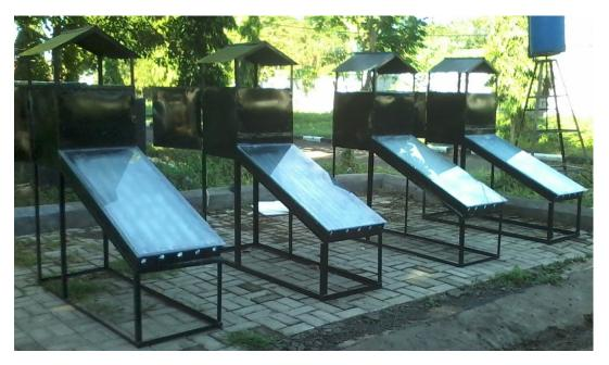
Figure 2: Shelf type of solar dryer with four fin types
