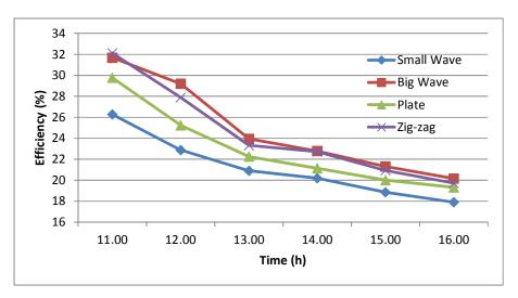
Figure 6: The influence of various fin types on solar dryer efficiency
