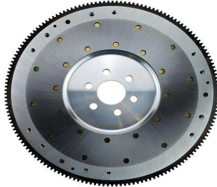
Gambar 2.9. Fly wheel/roda gila
