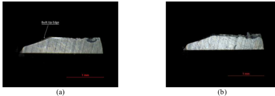
FIGURE 7. Wear of the tool under flood coolant drilling after (a) 15 th hole and (b) 37 th hole
