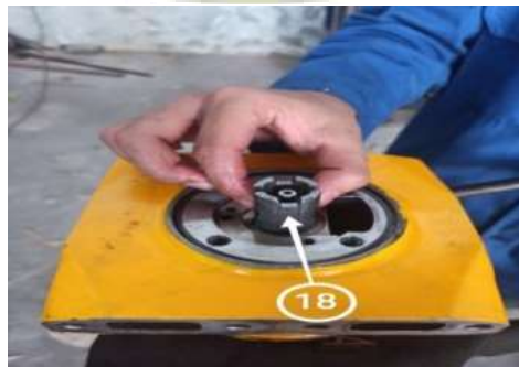
Gambar 3.5 Pemasangan Spacer Bearing
