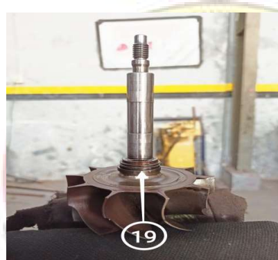
Gambar 4.11 Pelepasan Seal Piston Ring
