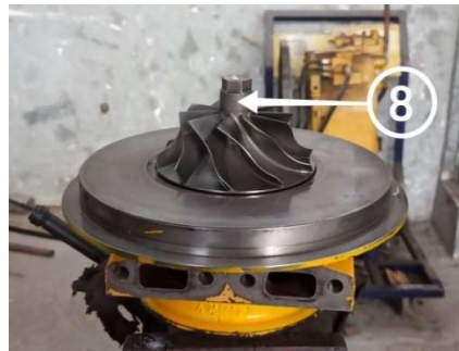
Gambar 4.5 Pelepasan Compressor Wheel
