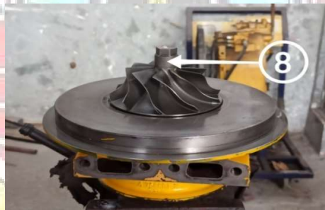
Gambar 2.3 Pelepasan Compressor Wheel
