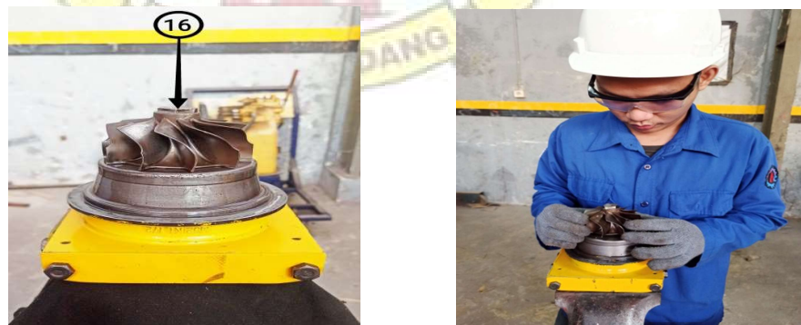
Gambar 4.16 Pemasangan Turbine Wheel
