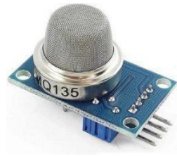
Gambar 2.7 Komponen sensor gas MQ-135
