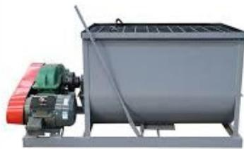
*Gambar 2. 3 Mesin mixing horizontal*
