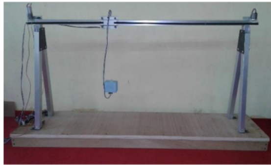
Figure 4. Experimental model of the gantry crane system
