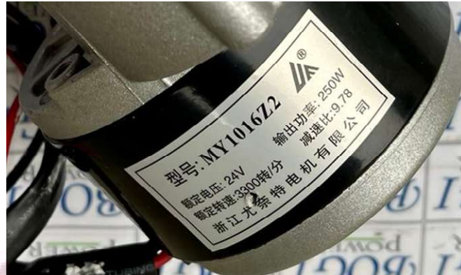
Nameplate Motor Listrik
