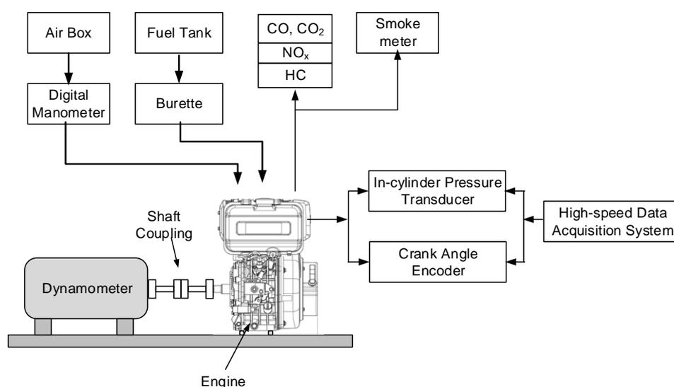
Figure 1 Schematic diagram of the engine test set-up
