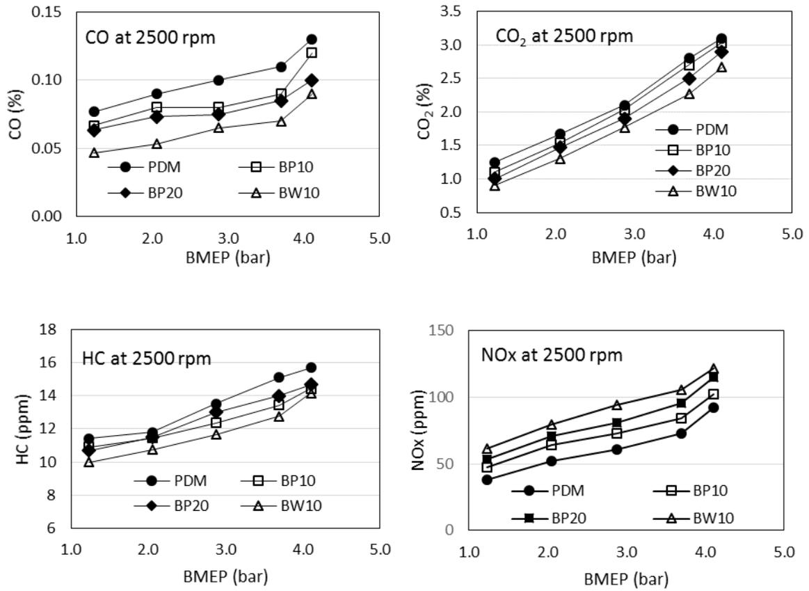
Figure 4 The variation of CO, CO<sub>2</sub>, HC, and NO<sub>x</sub> with engine BMEP at 2500 rpm engine speed
