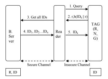
Figure 4. Extended Hash-lock Scheme
