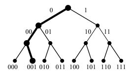
Figure 2. Concept of binary tree walking
