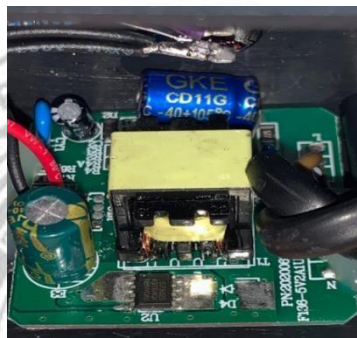
Gambar 3. 16 Perakitan Power Supply
