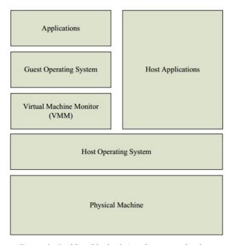
Figure 1. Building block of virtualization technology
